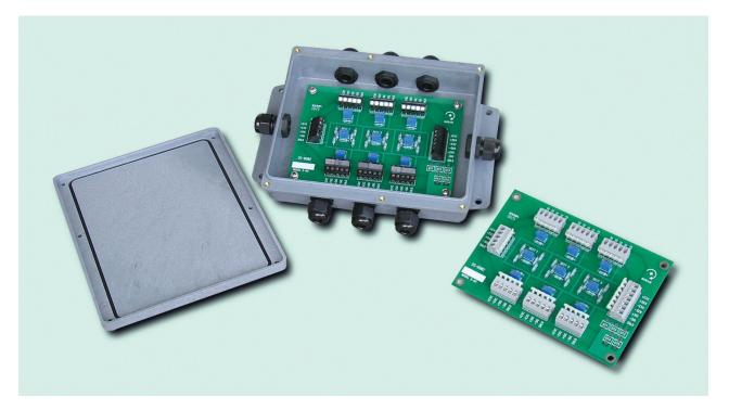
EVO Industries revolutionizes the truck scale summing box with a new series designed to overocome ALL of the problems with conventional summing boxes currently offered today! This box is the culmination of over 30 years' experience in designing truck scale summing boards and boxes.
